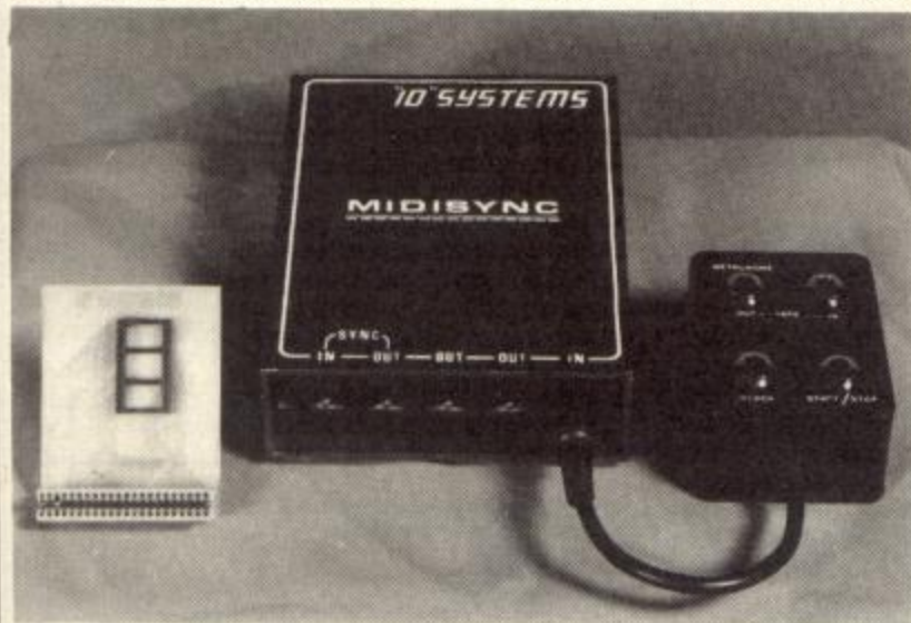
The MIDISYNC hardware in all its glory. It only fits comfortably onto the rubber-keyed Spectrum, so be prepared to buy an extension if you have a 'proper' keyboard. . . .
